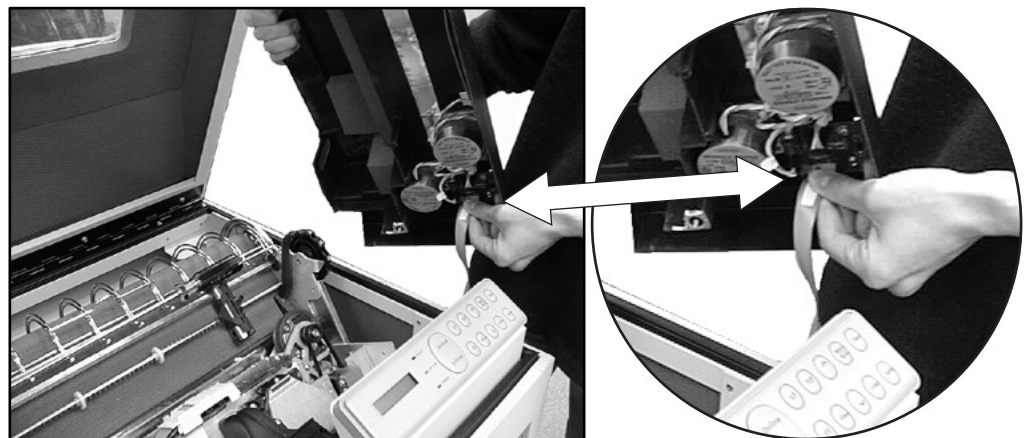
Figure 2. Unplugging Ribbon Drive Motor cable.
